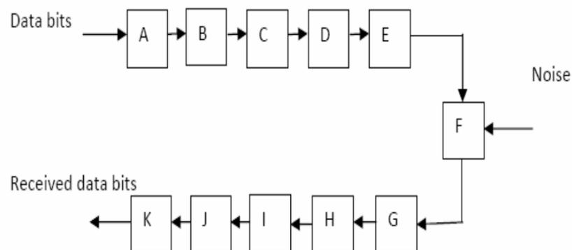
Digital Modulation : BPSK QPSK, QAM Turbo code rates : 1/3 SISO Decoder :Log-MAP Code Generator : {111, 101} Interleaver : pseudo random interleaver We measured the performance of the turbo coded OFDM through
