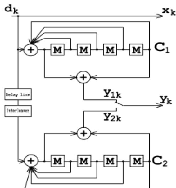
In the figure,  $M$  is a memory register. The delay line and interleaver force input bits  $d_k$  to appear in different sequences. At first iteration, the input sequence  $d_k$  appears at both outputs of the encoder,  $x_k$  and  $y_{1k}$  or  $y_{2k}$  due to
